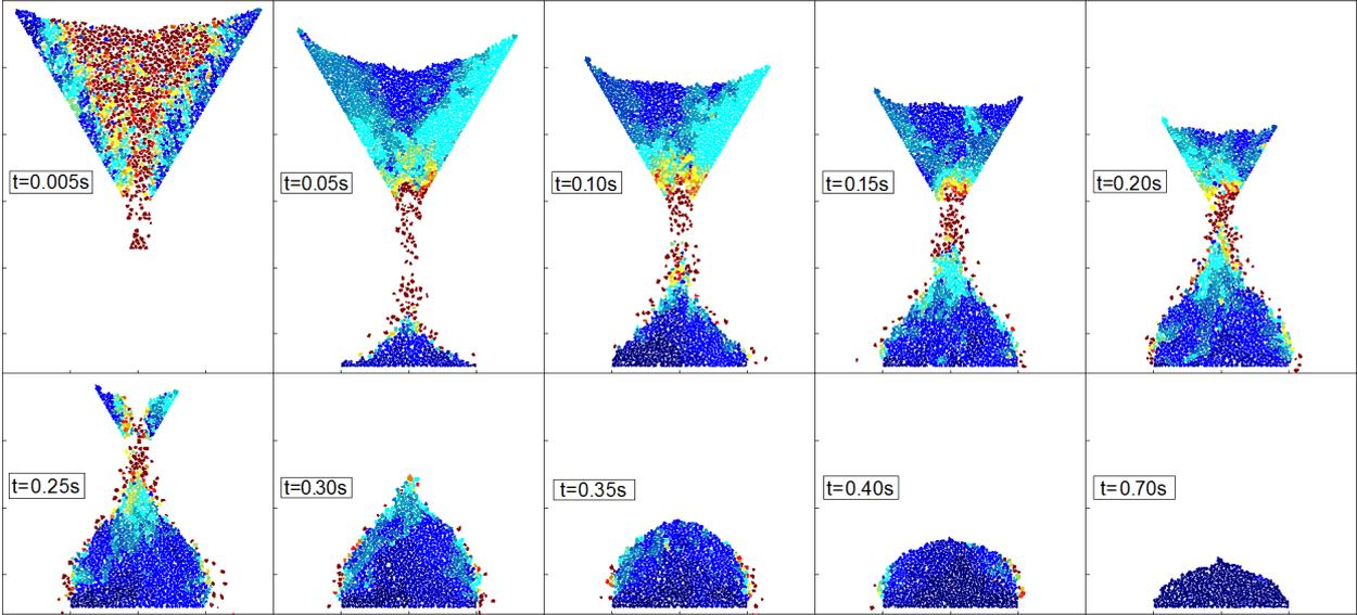
Fig. 7. Granular flow through the hopper and deposition (colour indicates velocity)
