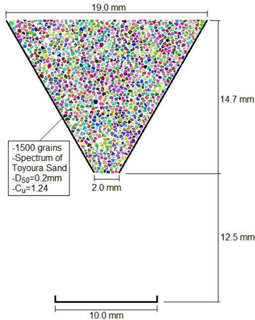
**Fig. 6.** Layout of the simulation
