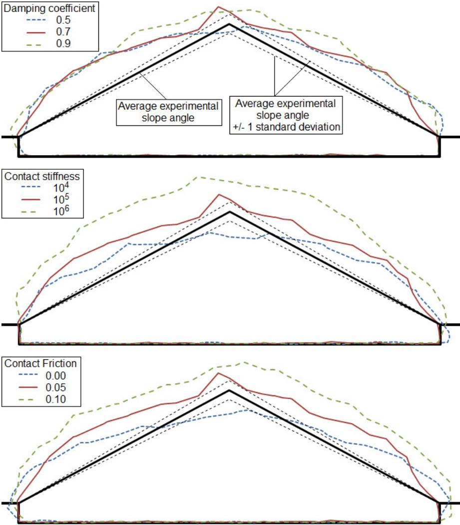
**Fig. 9.** Sensitivity study on the mechanical parameters of the simulation (Damping coefficient, contact stiffness, and contact friction coefficient)
