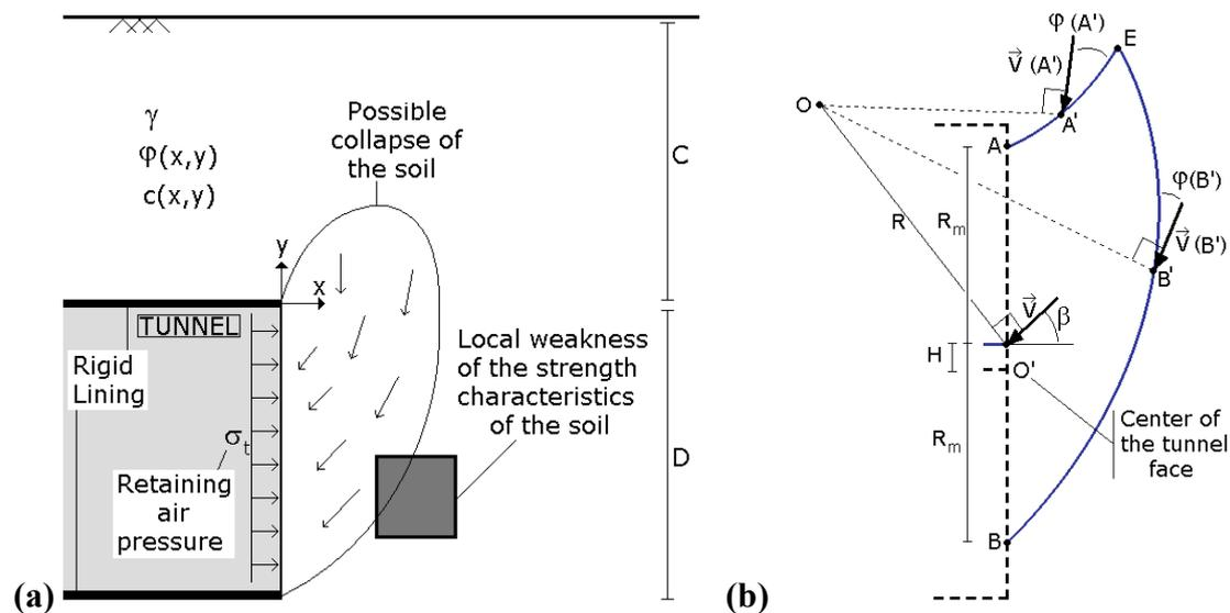
**Fig. 1: (a) Geometry of the problem and (b) definition of the four parameters governing the proposed failure mechanism ( $R$ ,  $\beta$ ,  $H$  and  $R_m$ )**
