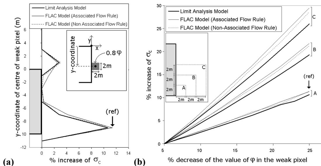
**Fig. 5: Impact of (a) square pixel location and (b) square pixel size and percent decrease of  $\phi$  inside the pixel, on  $\sigma_c$**
