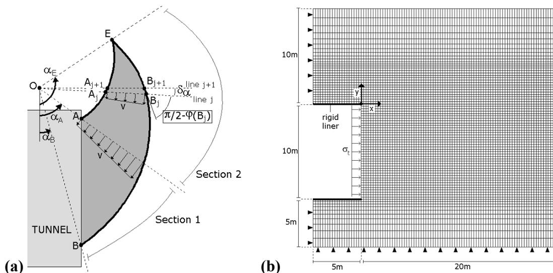
**Fig. 2: (a) Principle of generation of the proposed limit analysis model and (b) mesh of FLAC numerical model**
