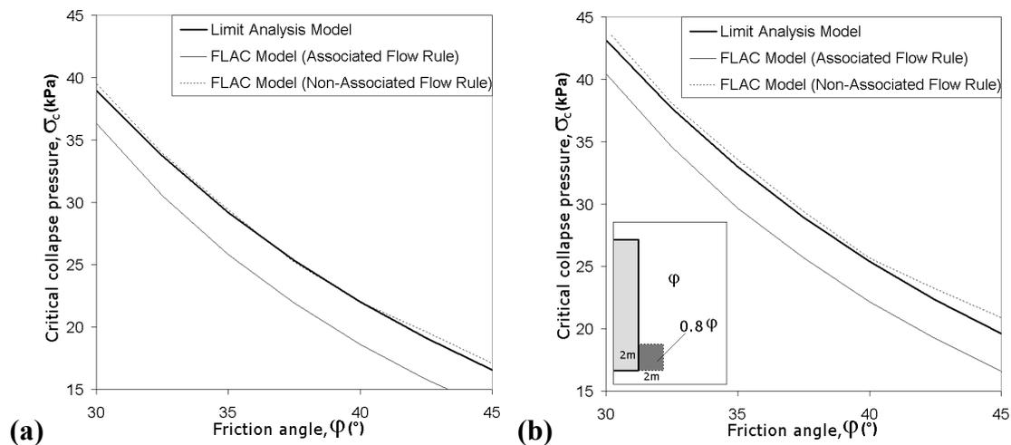
**Fig. 4: Critical collapse pressures provided by the proposed mechanism and FLAC model (with  $\psi=\phi$  and  $\psi=0$ ), for (a) a homogeneous sand and, (b) a local decrease of  $\phi$  by 20% in a 2m square pixel at the tunnel invert**
