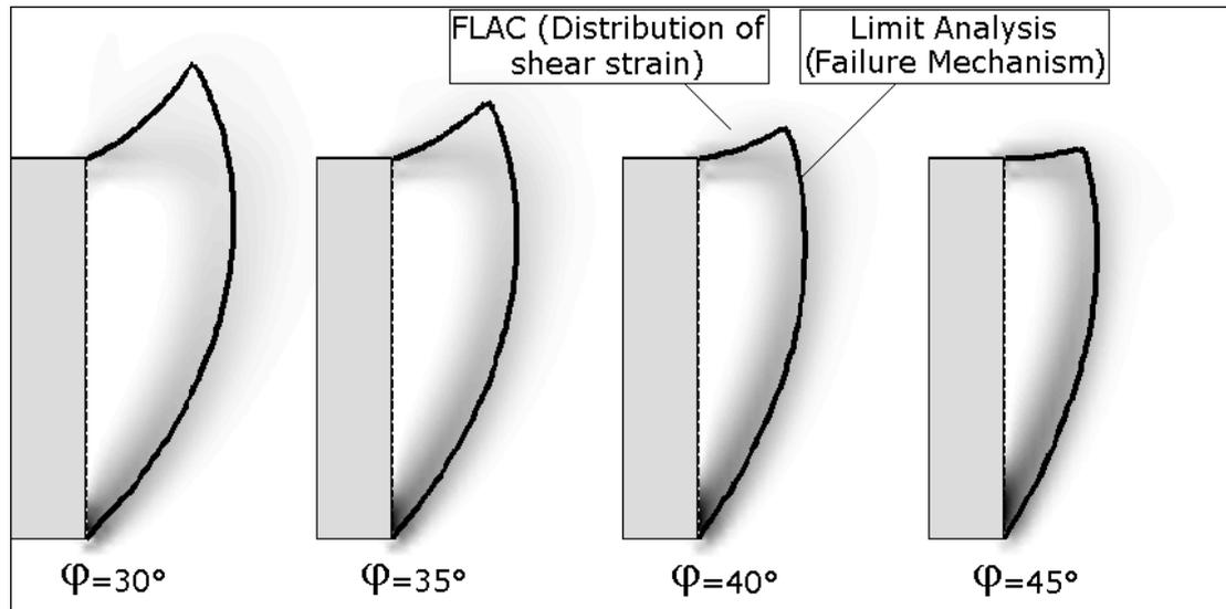
**Fig. 3: Comparison of the failure mechanism provided by the proposed model and the shear strain distributions provided by FLAC for an associated flow rule**
